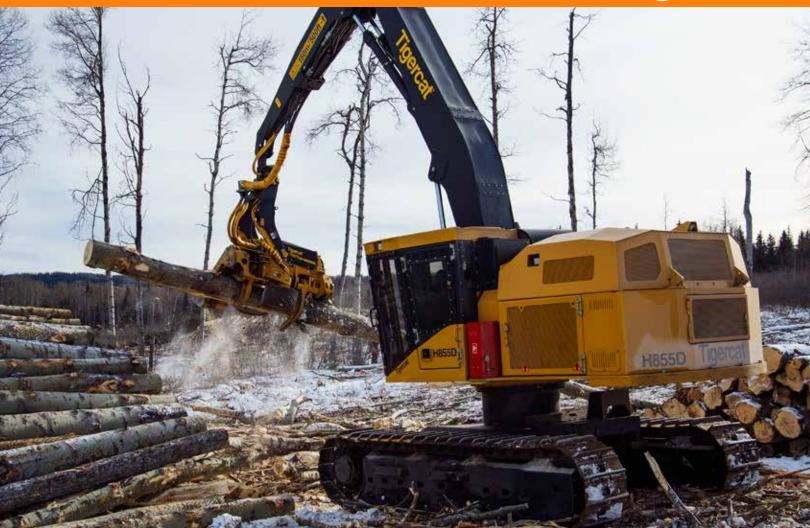
The Tigercat H855D series harvesters are durable, reliable and efficient. The carriers are designed for high performance harvesting, at-the-stump processing and roadside processing duties.
