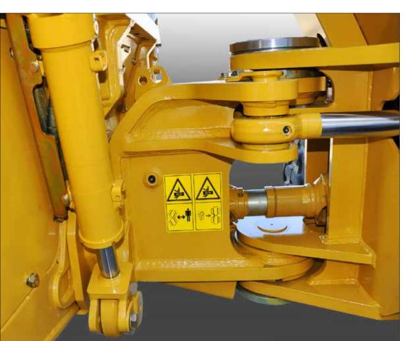
Tigercat forwarders are equipped with a unique centre section. The oscillation joint is situated on the wagon frame for high stability when turning, operating on slopes and loading with the crane at extension. The centre section is constructed with large pins and tapered roller bearings for low maintenance and long life.
