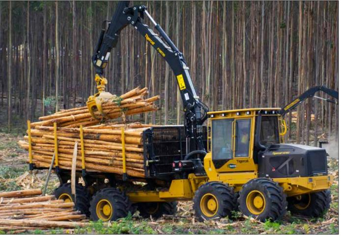
The bogie axles are equipped with a friction clutch differential lock or MDDL (multi disc differential lock). This allows the operator to engage and disengage the differential locks while the machine is moving for increased productivity.
