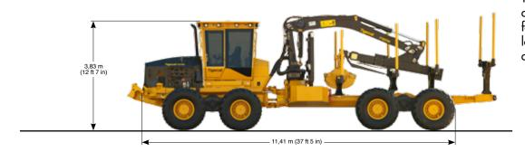
The 1075C is an extreme duty 20-tonne forwarder for final felling applications, long distance forwarding and scarifying applications.
