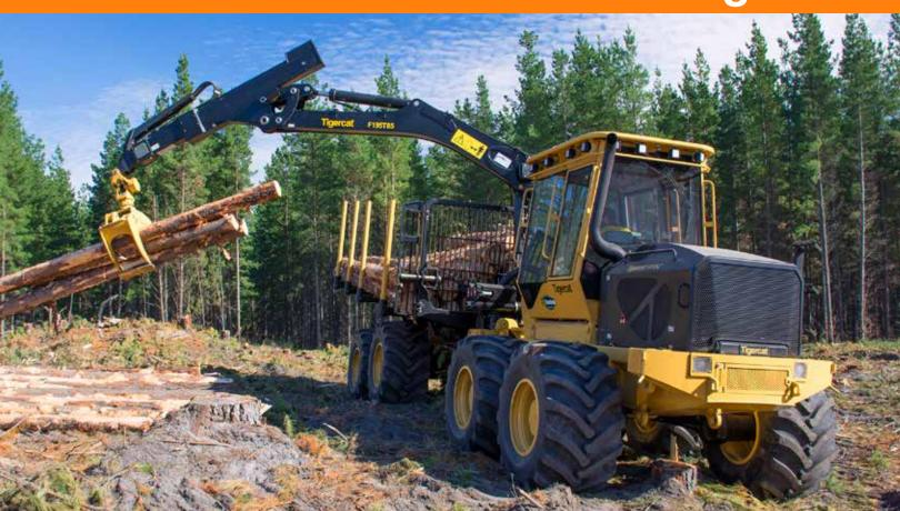
Tigercat forwarders, ranging in capacity from 14 to 25 tonne, are designed to achieve high production and lowest cost per tonne in the world's most demanding transporting applications.
