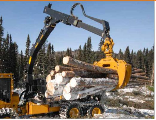
The Tigercat FG43 and FG53 grapples compliment the powerful Tigercat F195T85 crane with larger load areas for quicker cycles. Thick walled bushings, heavy duty Tigercat link, rotator and swing dampener with superior hose routing.
