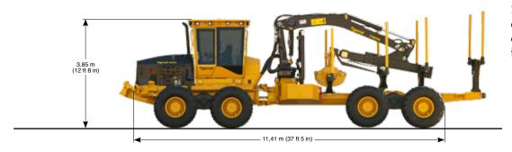
The 1085C is a severe duty 25-tonne forwarder built for extreme terrain and the most demanding, high production forwarding applications.
