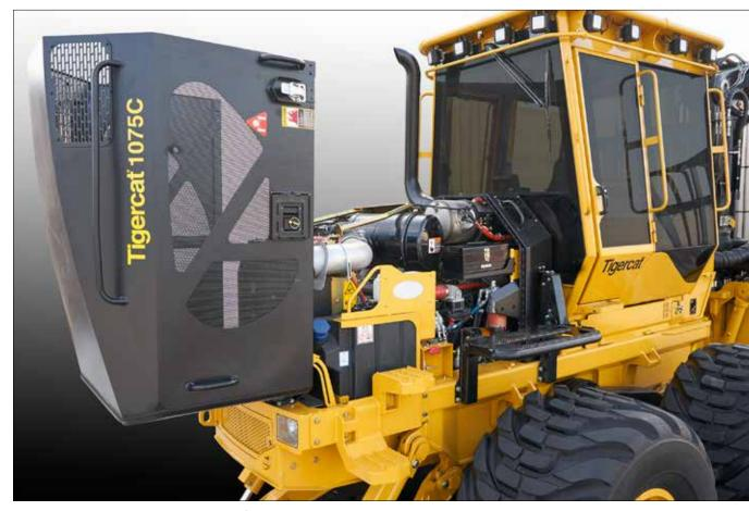
Excellent access to the engine and after treatment components. The strong steel tilting engine house cover protects the engine and cooling system components and acts as a work platform when opened up. No add on guarding is required.
