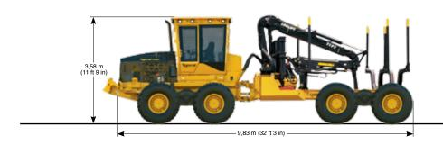
The 1055C is a heavy duty 14-tonne forwarder for selective felling, final felling and biomass applications.
