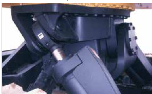
Massive pins and cylinders, thick steel plate and tapered roller bearings
