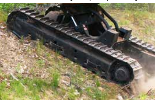
Long track frames and wide carbody for stability on slopes
