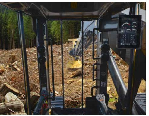
Excellent cab ergonomics and clear visibility to the track tips through the full length front window with narrow side posts.
