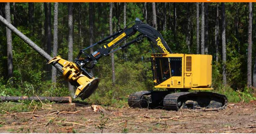
The Tigercat 822D feller buncher is designed for challenging thinning and final felling. Powerful lift capacity combined with tight-tuck boom geometry minimizes site impact in selective felling applications.
